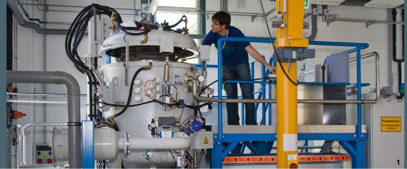
1 R&D furnace with a special heat-exchanger unit under the crucible bottom at the Fraunhofer THM in Freiberg.
